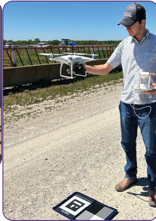
DJI Phantom 4 with NDVI camera (Left) being launched by visiting student (Middle) at Mound Valley to measure forage biomass in 14 pastures (Right).
