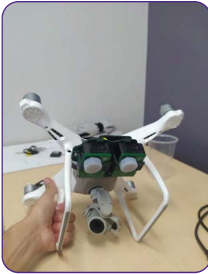
DJI Phantom 4 with NDVI camera (Left) being launched by visiting student (Middle) at Mound Valley to measure forage biomass in 14 pastures (Right).
